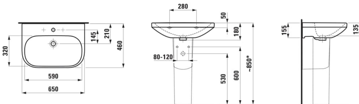
\* = Effective height must be fixed according to the height of the pedestal.
