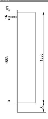
X = The exact hight must be set during installation.
